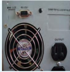
The RS-232 communication port and SNMP slot offered automatic shutdown with software control
