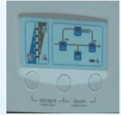
Designed with pressing both switches to start or stop the UPS to avoid touch by mistake
